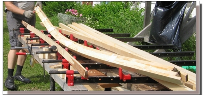
Gluing of birch for a flight of stairs we did last summer. The work was simply based on the method of the clamps being fastened to table so that an arc was to be formed. Pine and fir can be arched to a remarkable extent.
